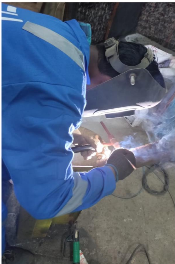
Argon welding set-up
